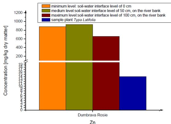
Fig. 8. The zinc concentration in the bulrush plant type, in one location: Dumbrava Rosie, downstream of Piatra Neamt city
